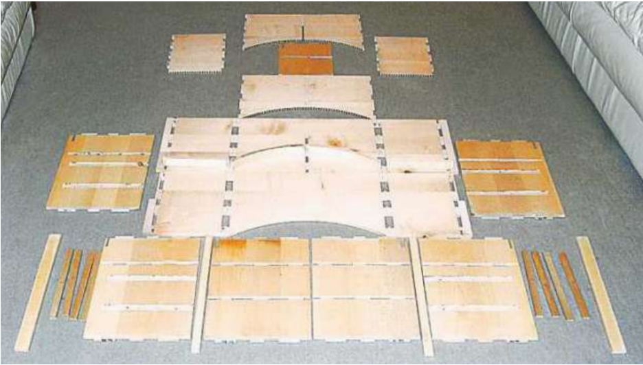
▲ Pic 20 Runners, drawers and dividers: all the pieces of the bureau's pigeon holes laid out ready for assembly
